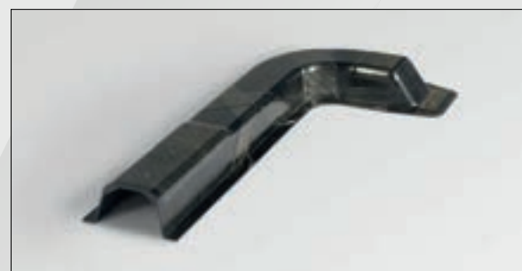
Multi-thickness demonstrator (optimised for 0% scrap)
