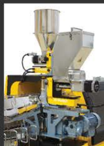
Side Feeder Gravimetric Hopper with Double-Screw
