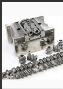
Extruder Barrel Module and Screw Elements
