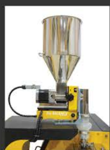
Main Feeder Gravimetric Hopper with Single-Screw
