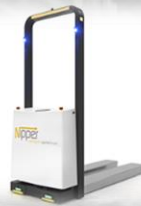
Autonomous drive fork-type transport robot
