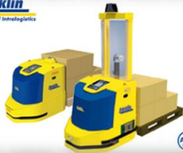
Autonomous drive fork-type transport robot
